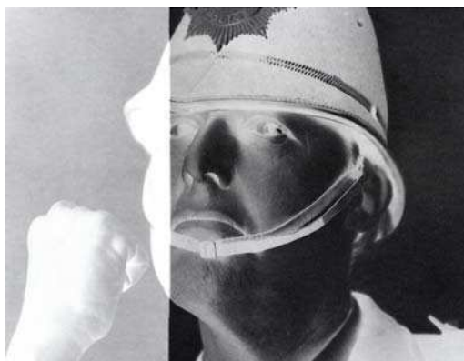
Figure 32.7 Processing faults. (Top) Dark, crescent-shaped kink marks. (Center) Underdeveloped clear patch, where this part of the film remained in contact with another. (Bottom) All negatives throughout the film show part of the picture pale. The cause is probably insufficient developer in the tank.
